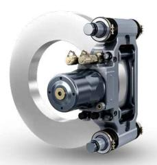
Among other things, Knorr-Bremse manufactures hydraulic brake calipers for high-speed trains.
